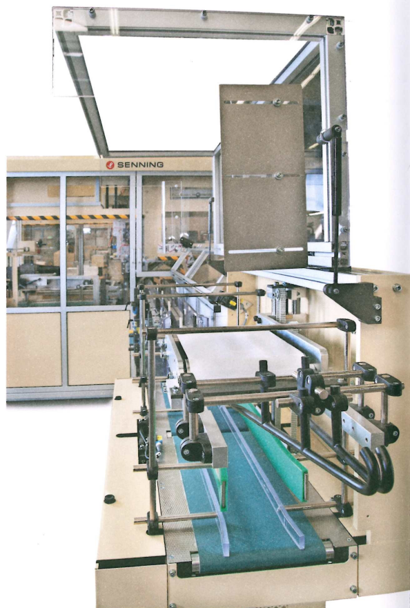
Special feature: inline take-over with "guide runners" for an ideal inline transfer
